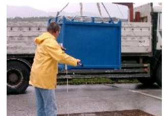
Drop test for a filled steel box from a height of 1,20 m
