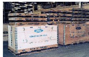
Ford also saves space thanks to the RePak T's 1:5 collapsibility ratio
