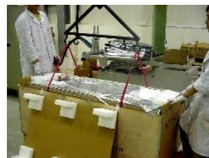
PE-foam with strong cushioning ability is next to be put on top before lid is assembled
